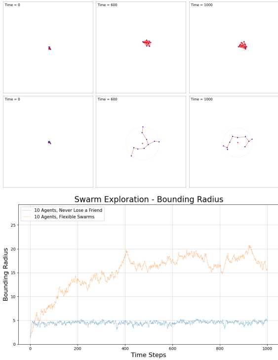
Fig. 7: The influence of flexibility on the swarm size over time (from left to right). The figure shows two rows of images: the top row displays swarm exploration under the “Never Lose a Friend” algorithm, while the bottom row illustrates exploration under the “Flexible Swarms” algorithm. The comparative bounding radius graph illustrates the difference between the two algorithms throughout the entire scenario.
